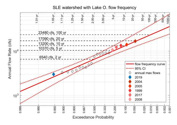
Figure 5. Exceedance probability of freshwater inflow from all sources to the St. Lucie Estuary based on data from 1999 to present. The various 'diamonds' illustrate maximum annual flows for all years in the record, with blue (2019) being the lowest maximum flow and the various red (2004, 2005, 1999, 2017, and 2008) being the highest five maximum flows.
