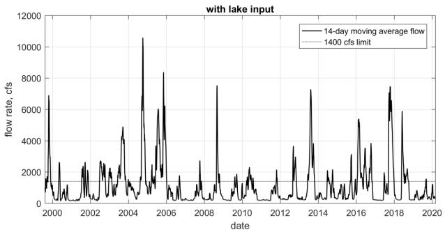
Figure 3. 14-day running average of total freshwater flow input to SLE, including groundwater and discharges from Lake O, for the period between July 1999 and March 2020.
