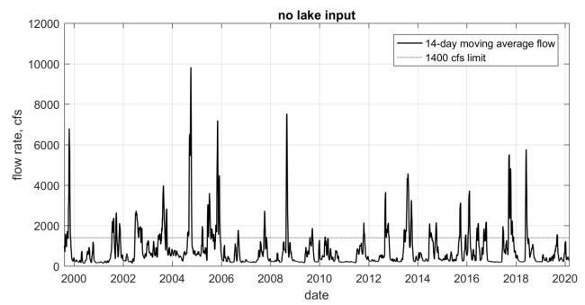
Figure 4. 14-day running average of freshwater flow input to SLE, including groundwater, but with discharges from Lake O removed, for the period between July 1999 and March 2020.
