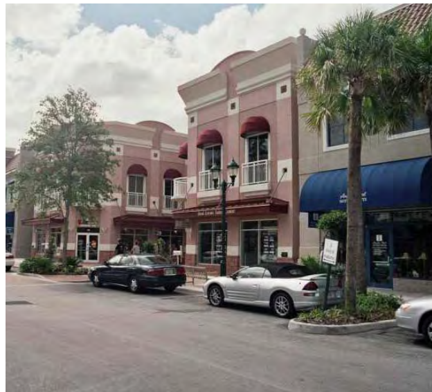
On Street Parking with Planted Bulb-Outs Buildings Set at Sidewalk as Integral Part of Streetscape
